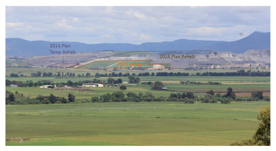
**Figure 3.** View of 2013 rehabilitation at MTW South Pit North. Rehab areas planned to be rehabilitated during 2014 are also shown. Vegetative cover will be established on a small area of temporary rehabilitation during 2014. Final rehabilitation cannot be completed in this area due to the location of maintenance infrastructure. Photo taken from Hambeldon Hill, Singleton.
