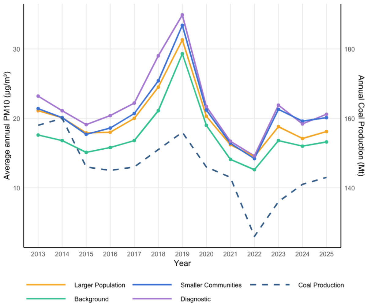
Figure 3-9: Comparison of Hunter Valley coal production data and UHAQMN annual average PM 10 concentrations
